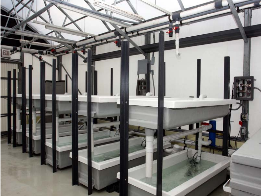
Figure 1: Experimental systems in use at the University of Miami. The top tank in each system is for experimental incubations, while the lower tank is the temperature regulation sump.
