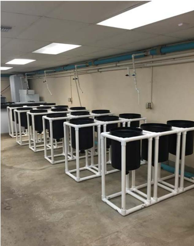
**Figure 3: 18 -tank flow through system used for stone crab larval rearing.**
