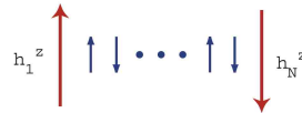
Figure 4.2: Antiparallel boundary fields (big, red) are compatible with antiferromagnetic alignment of spins (small, blue)
