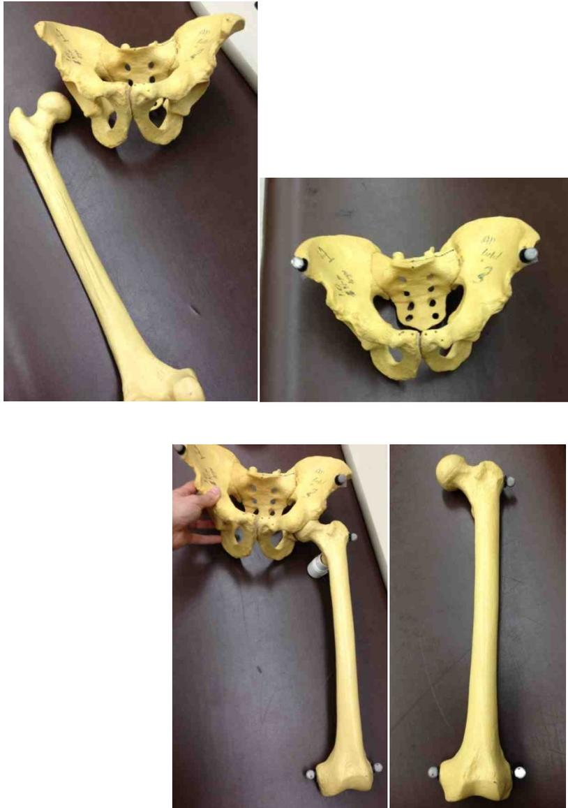
Markers are placed on the same bony landmarks as the human trial. The pelvis and femur were moved through the capture space by hand to simulate a gait trial. The hip joint was held together by hand, and the femur was swung in a pendulum pattern similar to a gait pattern.
